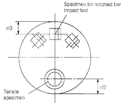
Figure 2 Sampling of steel bars, forgings and castings
