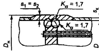
$$b_1 = \frac{D_H - D}{2}; R_1 = \frac{D_H + D}{4}; h_1 = s_p;$$
