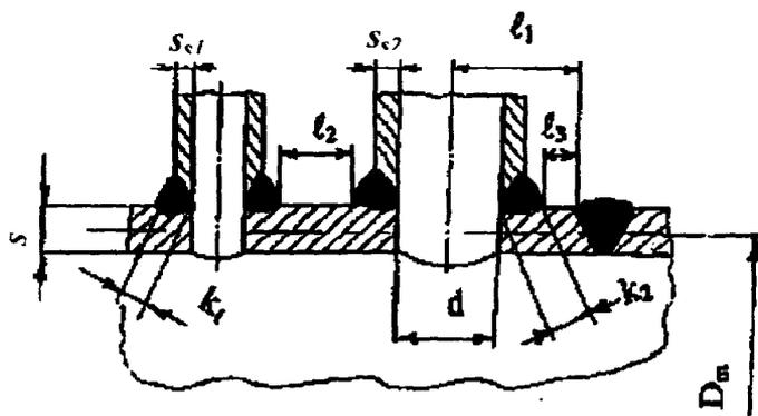
$$\ell_3 \geq \max(3k_2; 3s_{s2}); \ell_1 \geq 0,9 d; \ell_2 \geq \max(3k_2; 3s_{s2})$$
